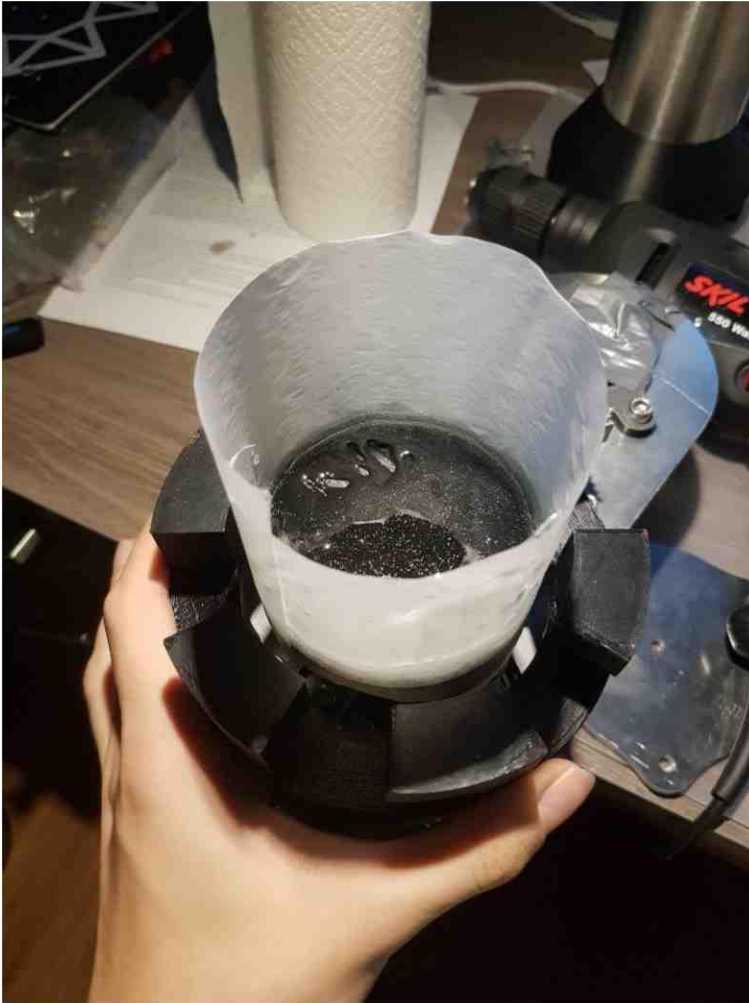
Figure 18 - Molding the piston head
