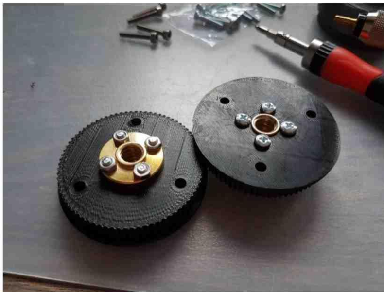
Figure 15 - Lead screw nuts inserted into ABS timing belt pulley
