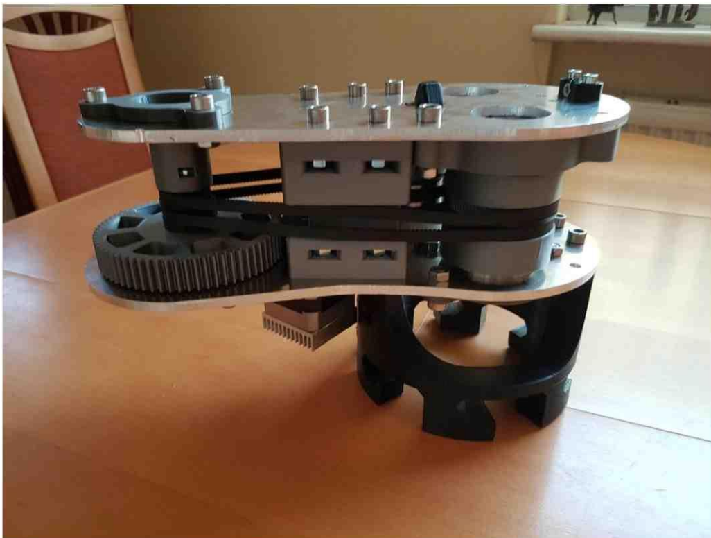
Figure 17 - Almost fully assembled extruder
