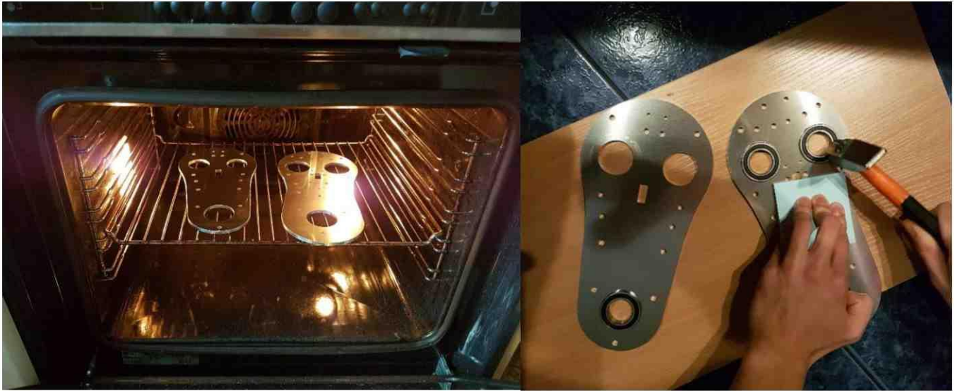
Figure 14 - Heating the aluminum frame plates to press the bearings into them
