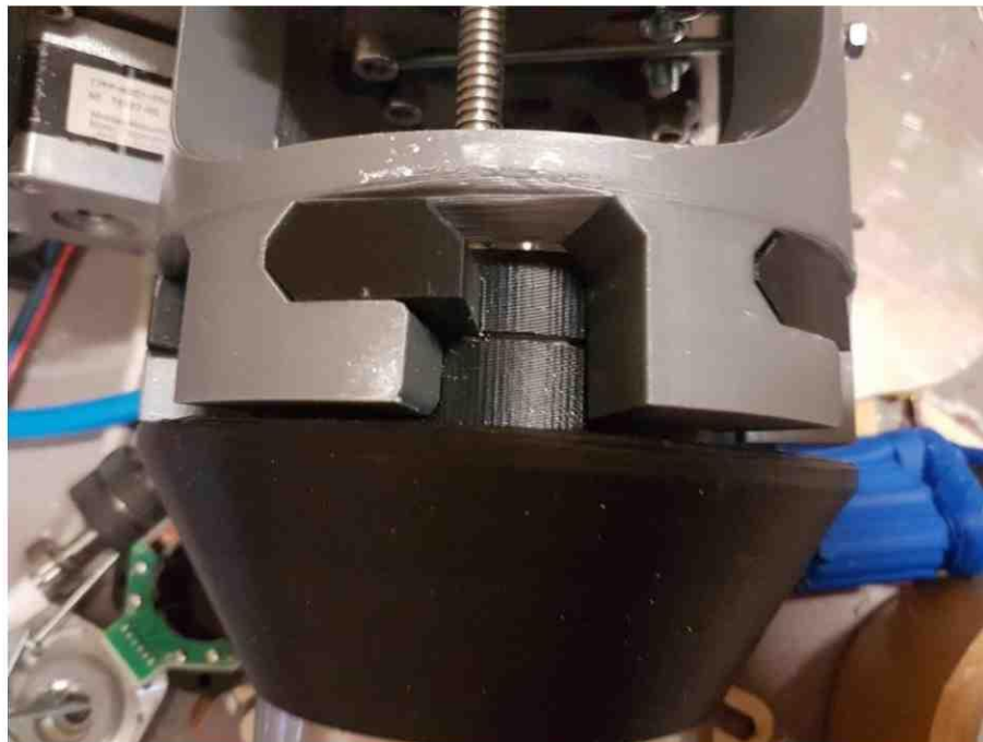
Figure 23 - the other part of the top pipe mount split in between the layers
