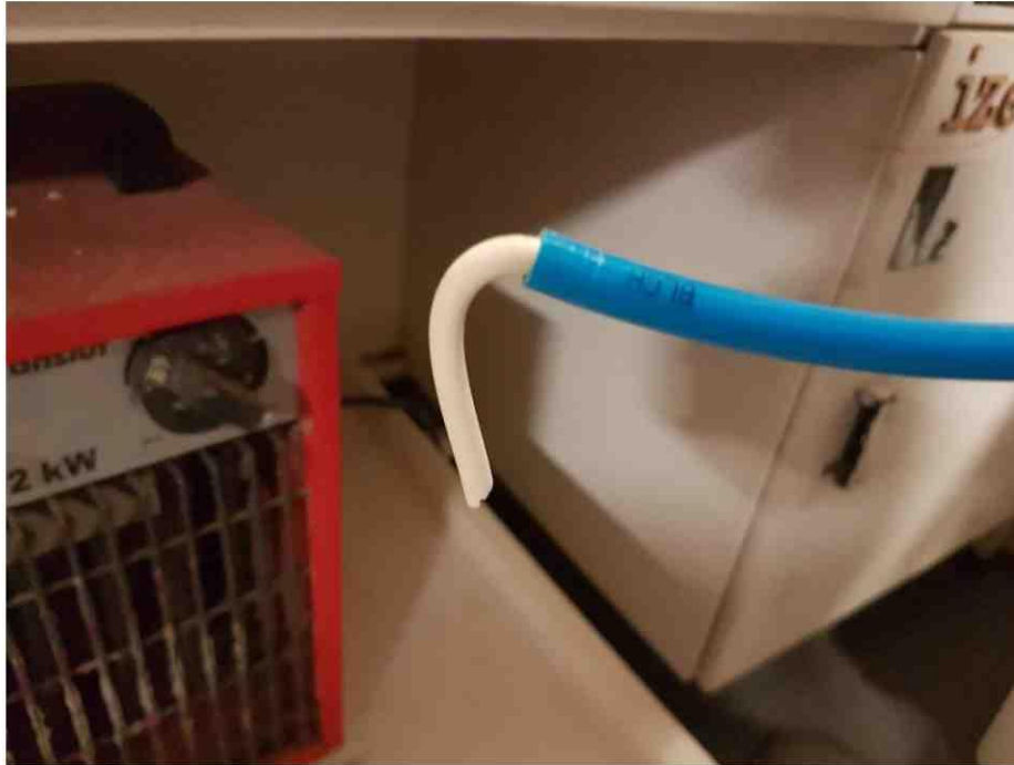
Figure 22 - clay being extruded by the actuated piston
