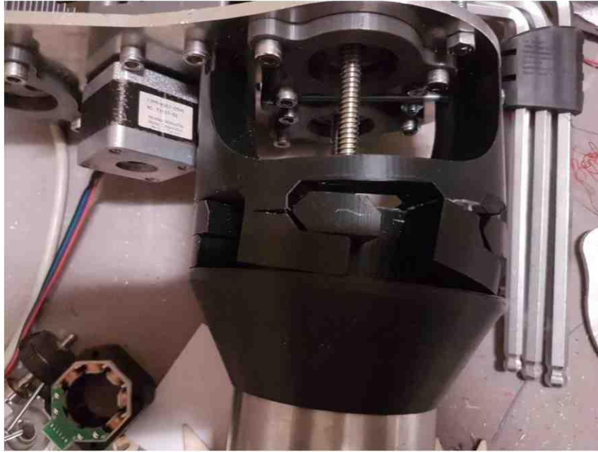
Figure 21 - top pipe mount split in between layers
