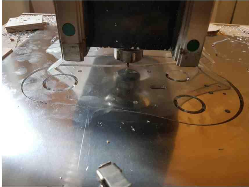
Figure 11 - The bottom frame plate just after being CNC machined
